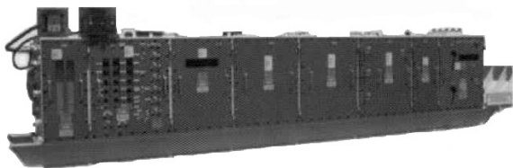
Example of a longwall controller box
